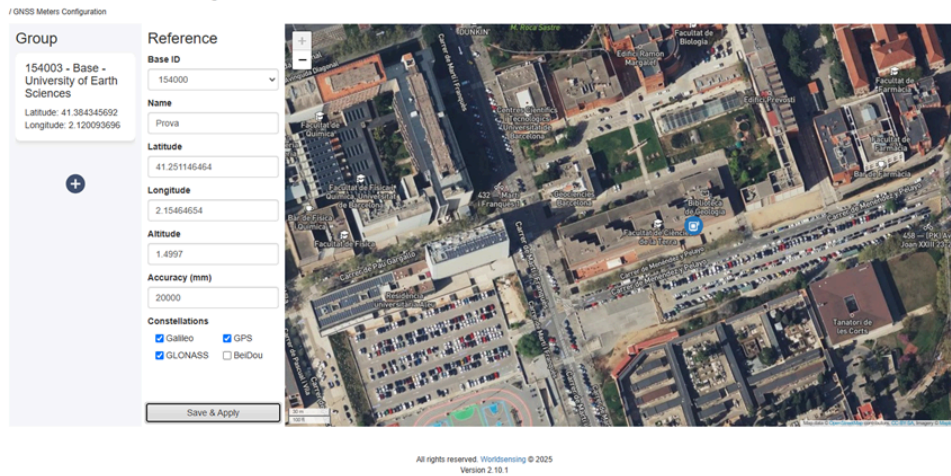
Figure 21: Creating a group on the GNSS Meters Configuration.
