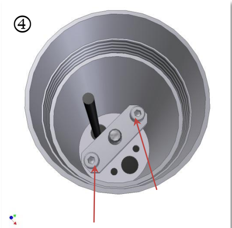
Extract the plate removing the two screws with allen key nr.3
