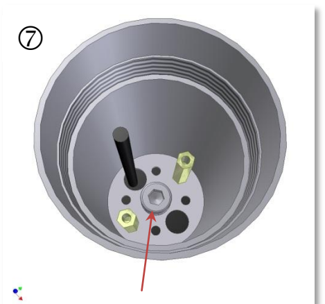
Once extracted the threaded rod, lock the M8x12 screw with the bonded washer - supplied with MEXID separately - for waterproofing.
