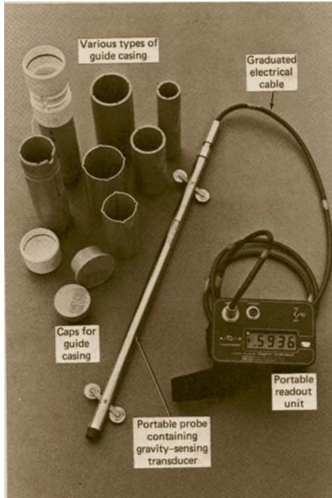
(a) Inclinometer system (after Slope Indicator Co., Seattle, WA)
