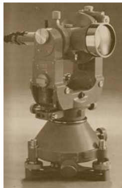
(a) Theodolite for measuring lateral movement (after Wild Heerbrugg, Inc.)
