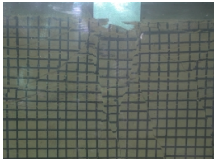
Figure 9. Failure pattern of the soft rock.
