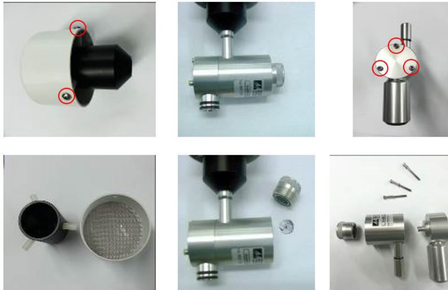
Figure 6-31 The TSP head and cyclone can be disassembled for cleaning.
