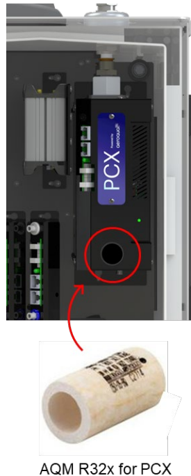
Figure 6-34 The PCX module requires an AQM R32
