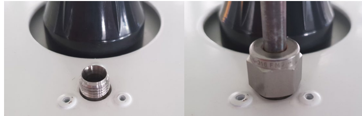
Figure 6-47 Gas inlet removed and attached to the 1/4" Swagelok fitting
