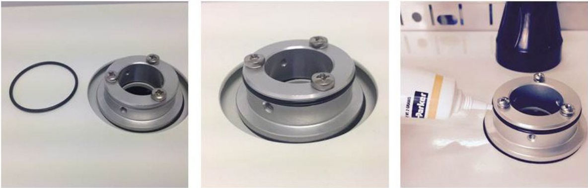
Figure 6-14 Add the O-ring and a small amount of lubricant.
