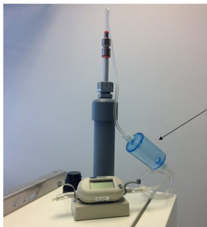
Figure 6-23 When measuring the flow on the Particle Profiler it is important to use the flow buffer chamber.
