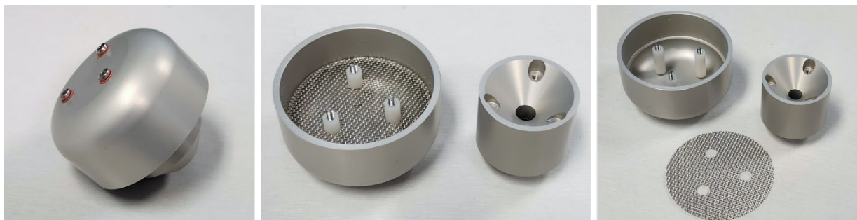
Figure 6-41 PCX TSP inlet disassembled for easy cleaning.
