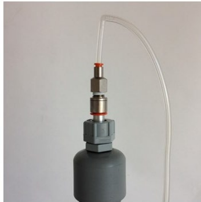
Figure 6-22 Positioning of the flow adapter when checking the flow rate on a Particle Profiler.
