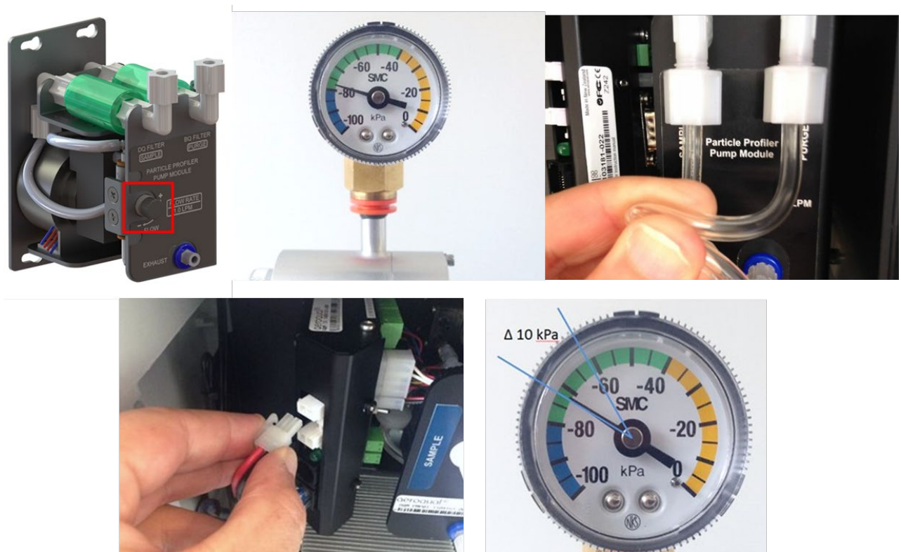
Figure 6-26 Adjust the sample valve, install vacuum gauge, and pinch purge flow tubing. Then remove power from module and time how long it takes vacuum pressure to drop by 10kPa.
