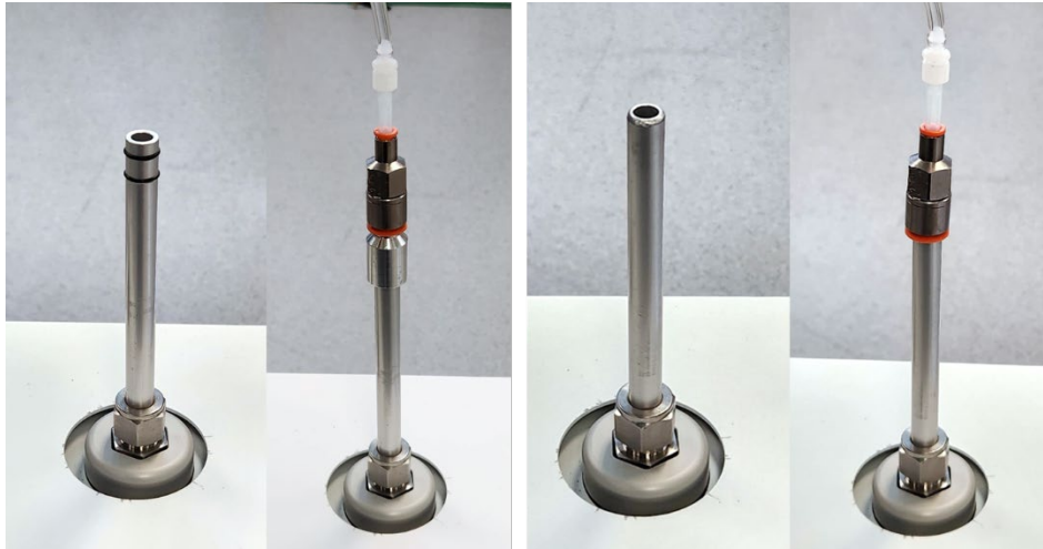
Figure 6-38 When checking the flow rate of the PCX replace the inlet with the adapter as shown. Left: Old inlet with O-rings that requires an extra adapter. Right: Current inlet without o-rings on the tube.
