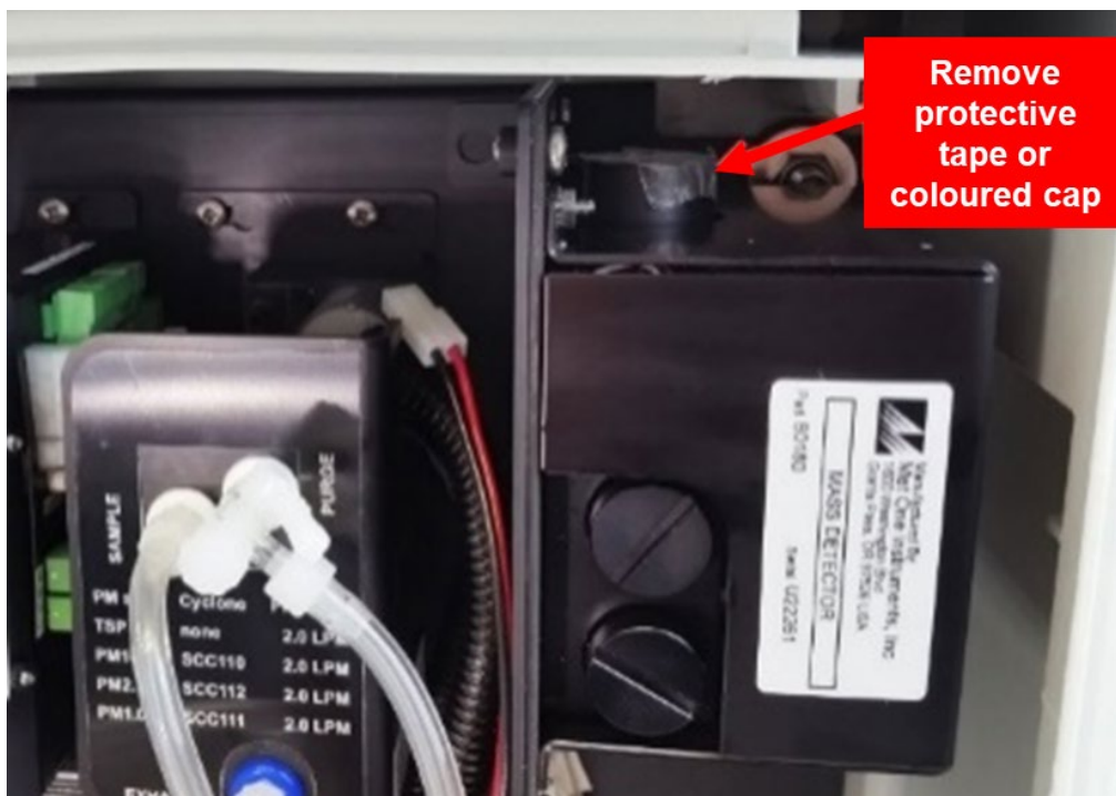
Figure 6-15 Remove the protective tape or cap from the PM inlet
