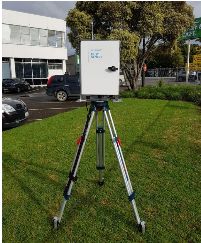
Figure 3-4 The monitor should be centered and level on the tripod
