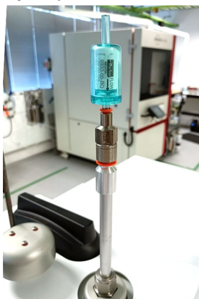
Figure 6-39 The zero filter can be attached to the inlet directly after removing the TSP inlet and O-rings
