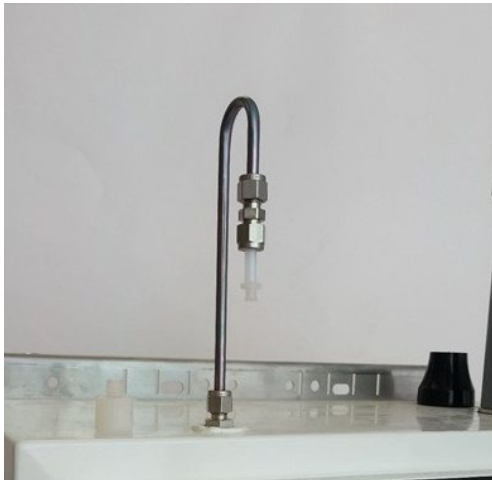
Figure 6-50 To measure the flow rate, remove the Kynar inlet filter and attach the inlet flow adaptor.
