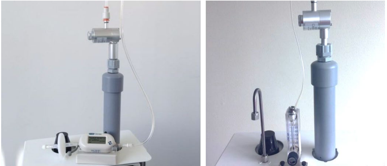
Figure 6-20 Flow meters connected to Particle Nephelometer inlet.
