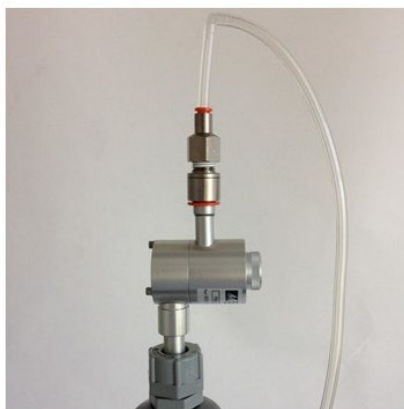
Figure 6-19 When checking the flow rate of the Particle Nephelometer place the flow measurement adaptor above the cyclone.
