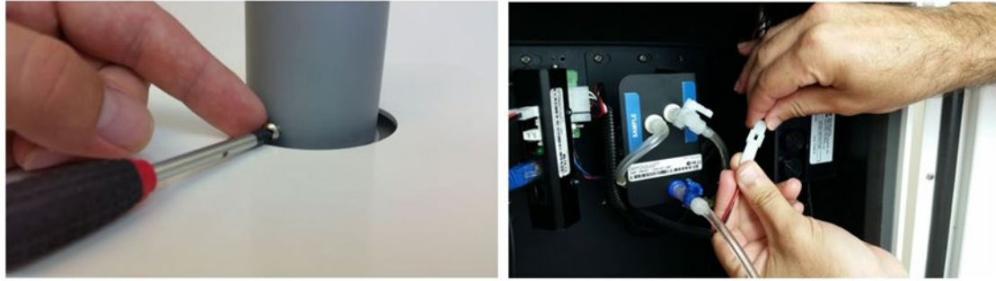
Figure 6-18 During field installation, secure the PM inlet using the retaining screws, then plug in the heater
