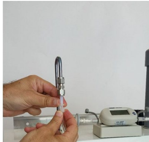
Figure 6-50 To measure the flow rate, remove the Kynar inlet filter and attach the inlet flow adaptor.
