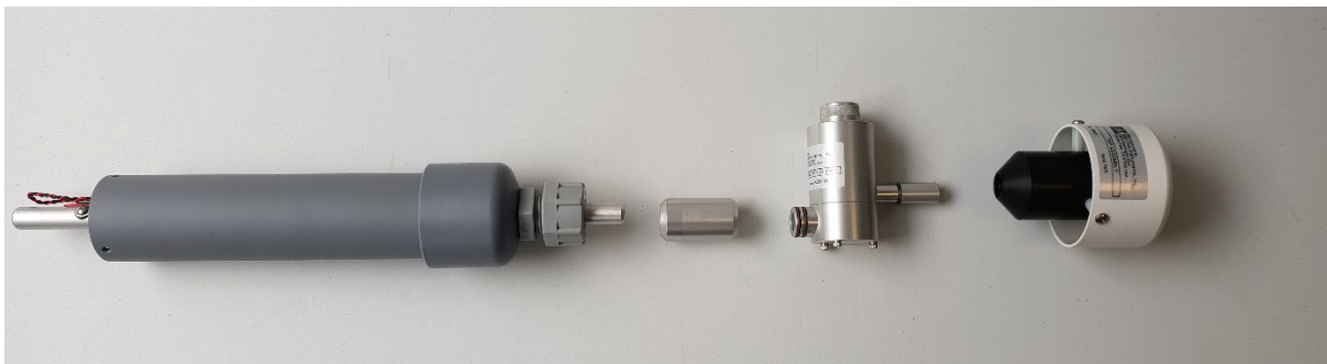
Figure 6-13 Particle sampling inlet parts including (L-R): inlet tube, cyclone adaptor, cyclone, TSP head.
