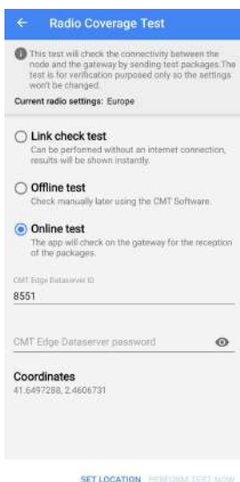
Radio signal coverage tests, including the Link Check test, and sample results
