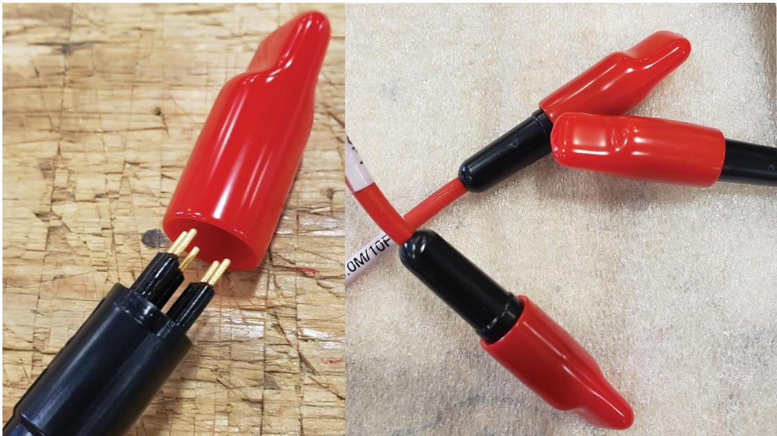
**FIGURE 2-11 ENSURE THE PROTECTIVE CAPS ARE PLACED ON THE CONNECTORS WHEN NOT IN USE**
