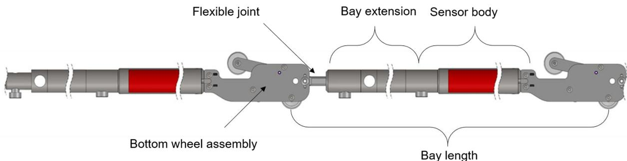
FIGURE 3-1 MEMS HORIZONTAL IPI ORIENTATION
