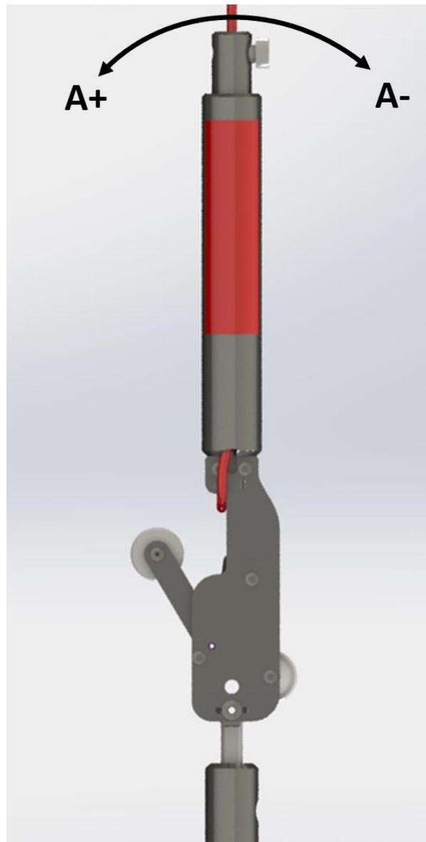
**FIGURE 2-8 MEMS IPI AXIS ORIENTATION**
