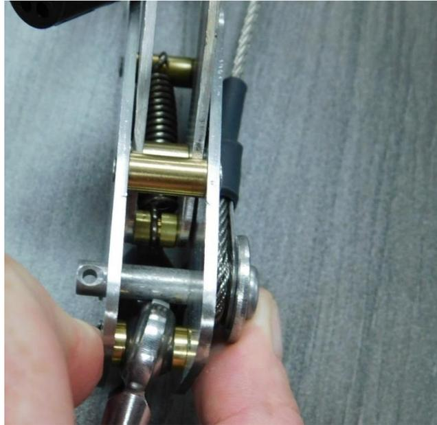
**FIGURE 2-6 PLACE WASHER AND INSERT CLEVIS PIN THROUGH WHEEL ASSEMBLY**
