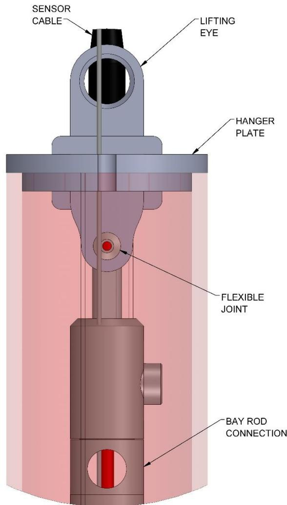
**FIGURE 2-2 COLLAR HANGAR SECURED TO TOP SENSOR**
