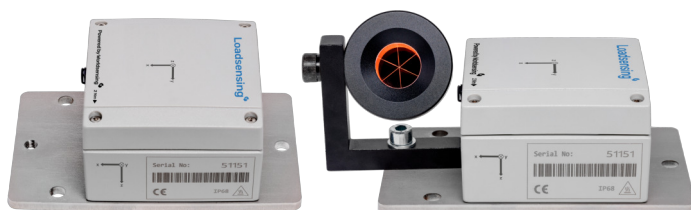
Fig. 3: Versatile horizontal surface mounting plate (LS-ACC-IN15-HP), recommended for both horizontal and vertical mounting. The plate has three clearance holes for M8 anchor rods and an M8 threaded hole available for installing a monitoring prism or a button head screw for precise levelling.
