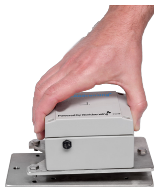
Fig. 6: The Tilt90-i mounted on a double plate for horizontal surface mounting (LS-ACC-IN15DP). This is suitable for applications that need avoid opening the casing during installation. The plate includes a threaded hole available for installing a monitoring prism or a button head screw for precise levelling.
