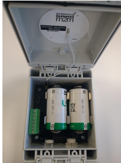
Figure 6: Unlike other LS-G6 nodes, there is no power switch in the Piconode
