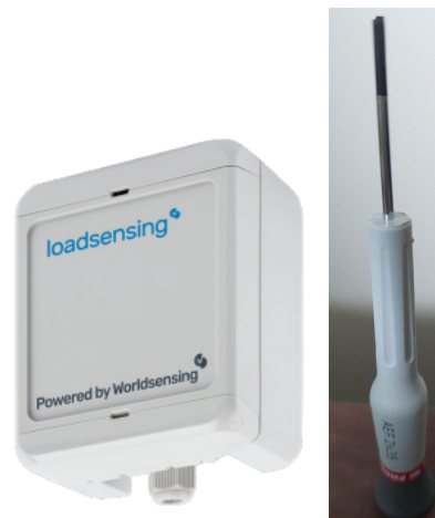
Figure 4: The Piconode can be opened making use of a 2-mm screwdriver
