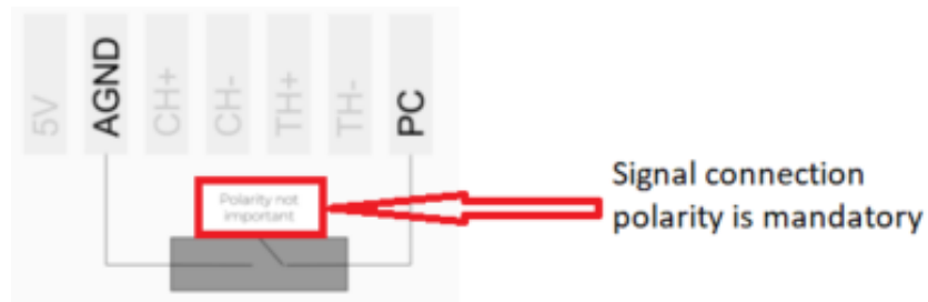
Figure 18: Wiring diagram for a pulse counter (open collector pulse)
