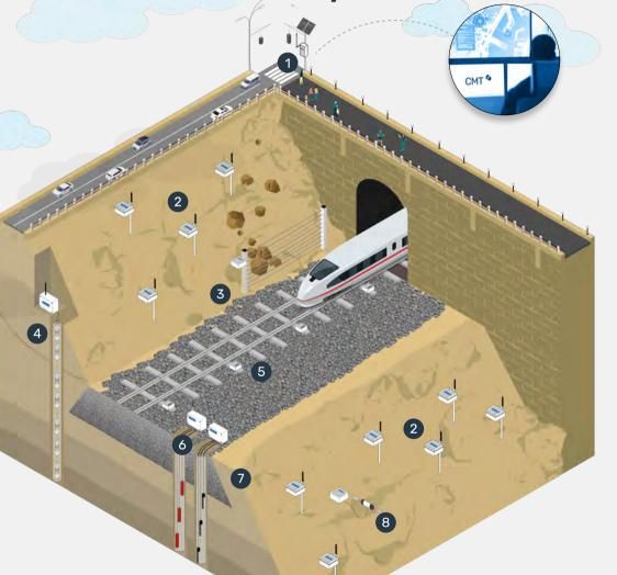
Remotely manage and monitor your network and all deployed devices either on-premise or through the cloud through a **Loadsensing gateway** sending data to the **Connectivity Management Tool (CMT)**. Integrate your data analytics software in CMT to create complete monitoring reports.
